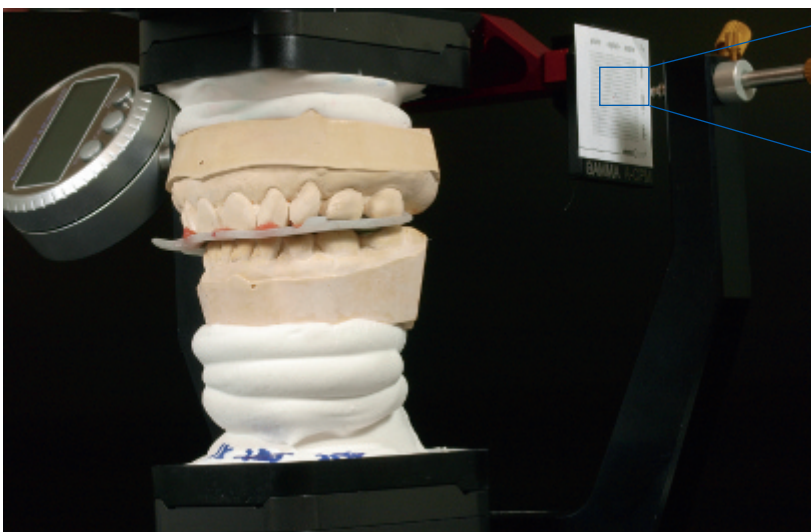
Fig 8 Positioning the models in the condylar position measuring instrument according to a centric bite record just obtained from the patient. Marking of the condylar position in red (see detail).
