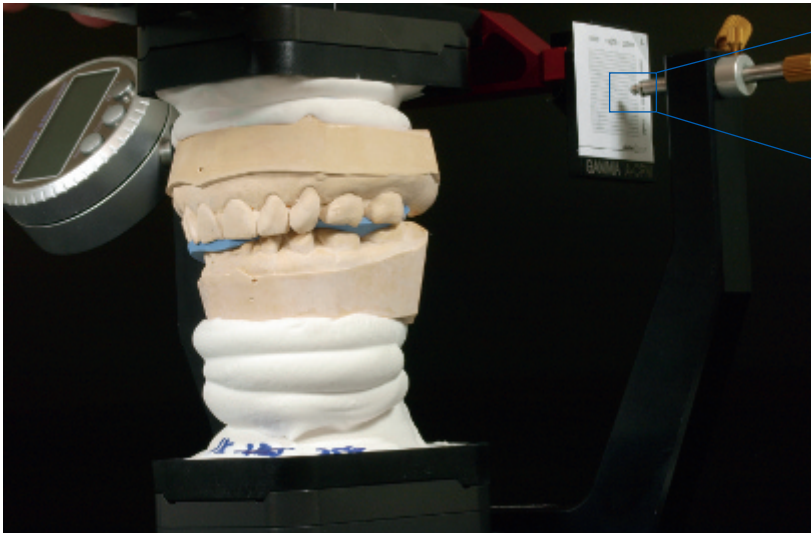
Fig 6 Transferring the models to the condylar position measuring instrument, positioning the models using a bite transfer template, marking of the condylar position in blue (see detail).
